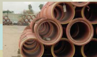
A stockpile of vitrified clay pipe, a standard pipe material used for local sewer projects.
